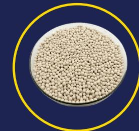
Zeolite molecular sieves are crystalline, highly porous materials, which belong to the class of aluminosilicates. This structure is formed by tetrahedras of  $(\text{AlO}_4)$  and  $(\text{SiO}_4)$ . SYLOBEAD® MS S 624 is a highly porous, binderless crystalline aluminosilicate in beaded form. The pore openings in the crystals have a diameter of approximately 5 Å.
