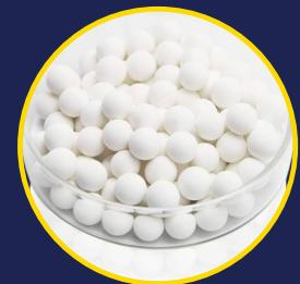
Activated alumina is made from aluminum hydroxide ( $\text{Al}_2\text{O}_3 \cdot n\text{H}_2\text{O}$ ) with dehydroxylating in a way that produces highly porous material. Activated alumina desiccant is a standard high performance, high porosity, high surface area activated alumina in beaded form. It has been specially designed to be used in the removal of water from gas and liquid streams and the removal of other polar compound.
