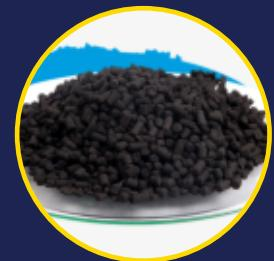
Activated carbon has appearance cylindrical extruded pellets with a grain diameter of approx. 3 mm. Activated carbon Type D47/3-PSA is produced by steam activation from de-ashed hard coal. It can be used for separation of hydrogen by pressure swing adsorption (PSA) technology from gases
