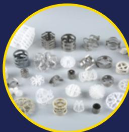
Random packing is used in separation columns, such as a distillation column, to increase surface area for vapor/liquid contact so that chemical separation is more efficient. In most chemical separation processes, vapor is driven upward in the column by heat and pressure while liquid falls downward under the force of gravity.
