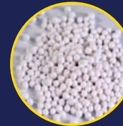
Activated alumina are made from aluminum hydroxide (Al<sub>2</sub>O<sub>3</sub>.nH<sub>2</sub>O) with dehydroxylating in a way that produces highly porous material. Activated alumina desiccant is a standard high performance, high porosity, high surface area activated alumina in beaded form. It has been specially designed to be used in the removal of moisture content from gas and liquid streams and the removal of other polar compound.
