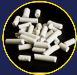
Desulfurizer Catalyst is an ultra-high porosity; high surface area zinc oxide adsorbent for the desulfurization of natural gas, off-gas, and other light hydrocarbon feed stocks in low temperature applications.
