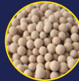
Zeolite molecular sieves are crystalline, highly porous materials, which belong to the class of aluminosilicates. These crystals are characterised by a three-dimensional pore system, with identical pores of precisely defined diameter. This structure is formed by tetrahedras of (AlO<sub>4</sub>) and (SiO<sub>4</sub>). For instance, the sodium form of zeolite A has a pore opening of approximately 4 Ångstrom (4 x 10<sup>-10</sup> m), called 4A molecular sieve.
